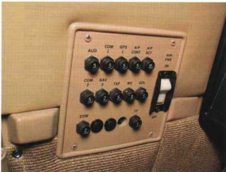
Renovated side panel circuit breaker panel.
