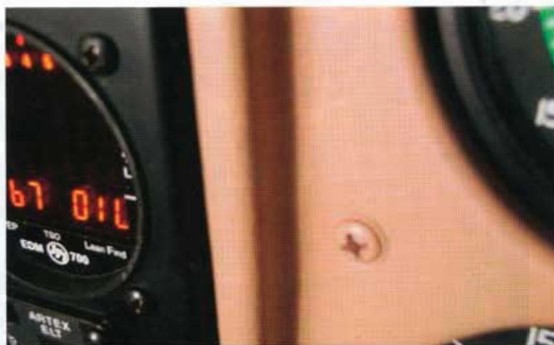
Painted finish screw and washer. Looks good, holds firmly and is easy to install and remove – wow!
