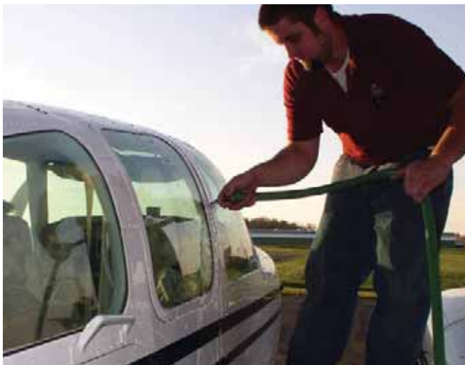
The ultimate leak test! Start at the bottom and work your way up.
